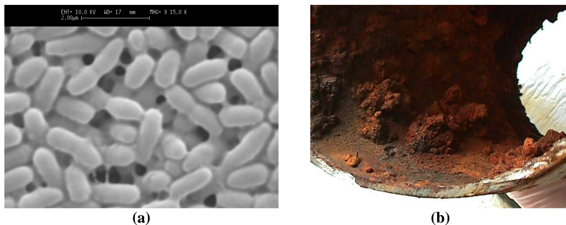
Figure 2.5 (a) Scanning electron microscopy (SEM) photomicrographs of 24 hours old biofilms formed by the opportunistic Gram-negative Burkholderia cepacia (isolated from laboratorial DWDS) evidencing the presence of an extracellular polymeric matrix ( \times 15000 magnification; bar = 2 \mu\text{m} ). (b) Ductile iron pipe section from a DWDS with biofilm and high amounts of corrosion products.
