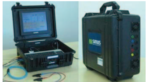
Fig. 1- Electric Power Quality Monitor in the transport case.
