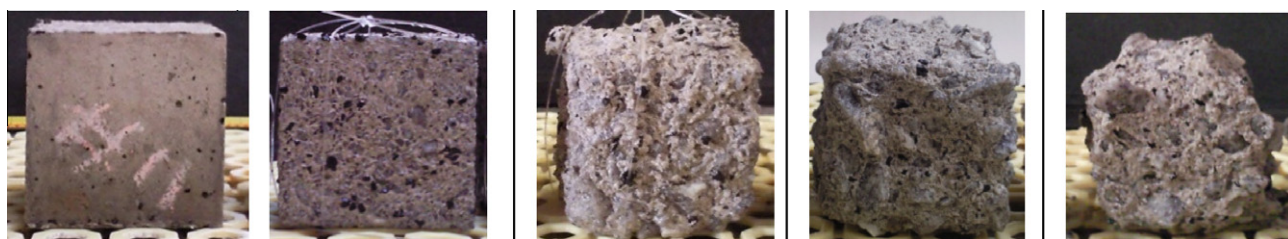
Fig. 8. Photos of concrete specimens with 5% rubber wastes and partial replacement of cement by 15% fly ash and by 15% metakaolin after immersion in sulphuric acid solution during 1, 3, 7, 14 and 28 days.
