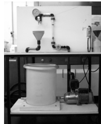
Figure 2 – Scheme of the equipment used for test the leaching of a sanitary brass tap in long term direct contact with water.
