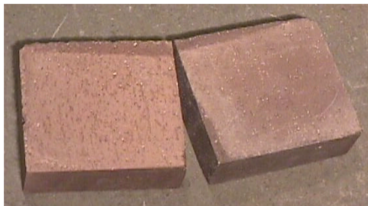
Figure 3.27 – Two half bricks used in the present testing program.
