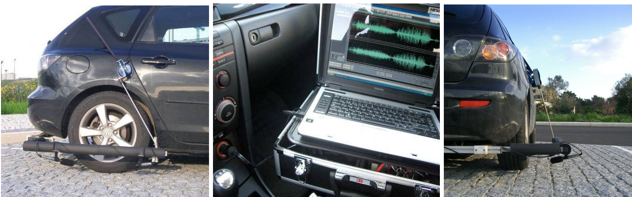
Figure 7 – Close proximity system used for the CPX tests
