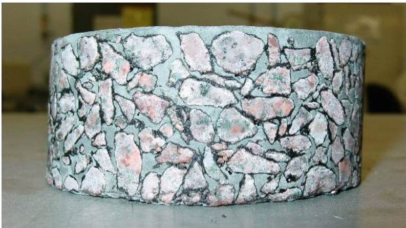
Figure 2. Core extracted from a typical grouted macadam slab
