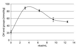
Figure 4. Hydroxyl groups in PET after treatment with different activities of the *T. lanuginosus* enzyme preparation. Error bars show the standard deviation of the measurement carried out in triplicate.
