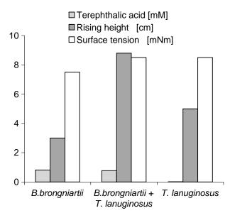
Figure 3. Hydrophilicity of PET samples and concurrent release of terephthalic acid after treatment with enzyme preparations from *B. brongniartii* (0.5 nKat mL<sup>-1</sup>) and *T. lanuginosus* (5 nKat mL<sup>-1</sup>) and a combination of both (0.5 nKat mL<sup>-1</sup> *B. brongniartii* and 5.0 nKat mL<sup>-1</sup> *T. lanuginosus*) The rising height and surface tension of control samples were 0 cm and 6.2 mNm, respectively.
