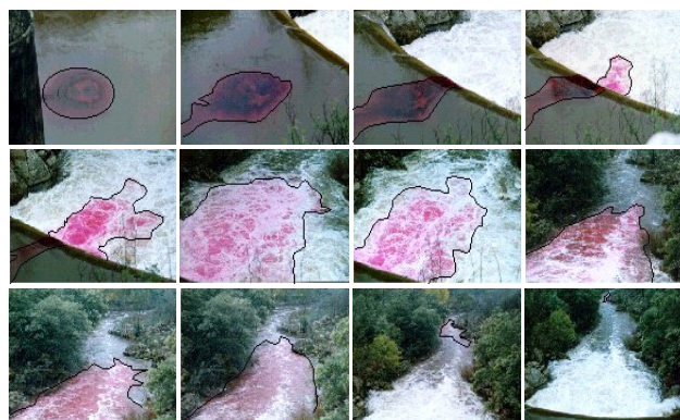
Fig.3: Rhodamine spreading after their injection (Mondego river at Caldas da Felgueira bridge)
