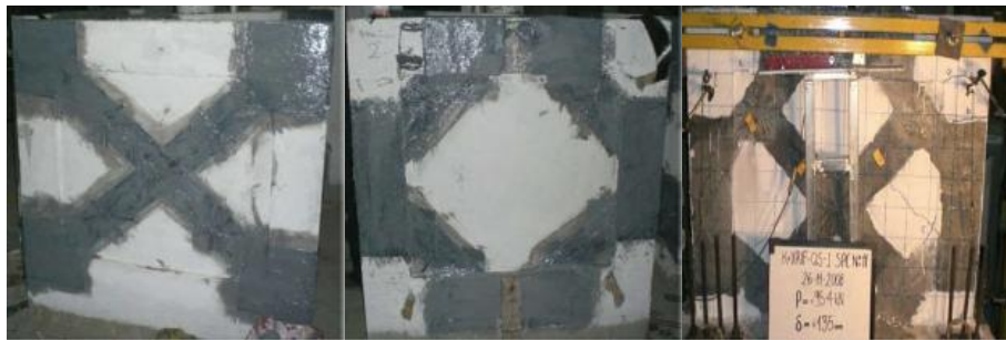
Figure 7 - Distinct retrofitting schemes on masonry infills by using carbon fibers reinforced materials [23]
