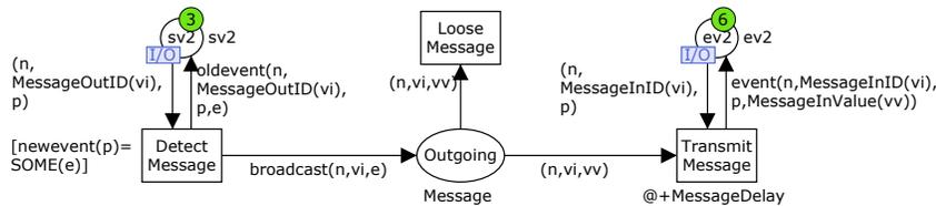
**Fig. 3** Environment assumptions expressed in the `CommunicationBus` module
