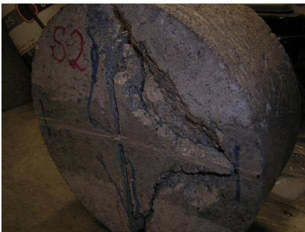
Fig. 5.12 – Specimen S2: semi-conical fracture surface (Master Thesis by João Lima)
