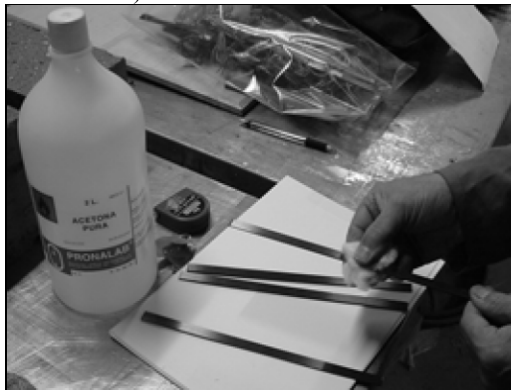
3) Cleaning of the laminates by acetone
