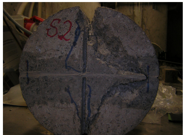
Fig. 5.12 – Specimen S2: semi-conical fracture surface (Master Thesis by João Lima)
