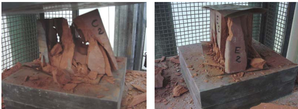
Figure 2-4 – Typical failure of the specimens tested along the X direction, half unit.
