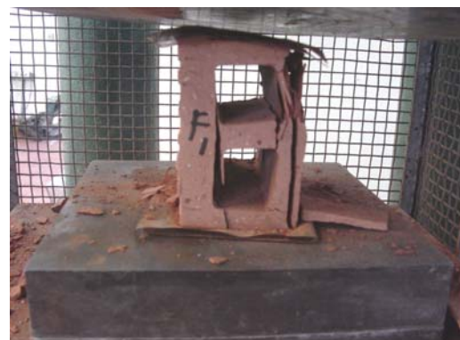
Figure 2-6 – Typical failure of the specimens tested along the Y direction, half unit.
