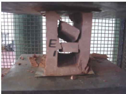
Figure 2-6 – Typical failure of the specimens tested along the Y direction, half unit.
