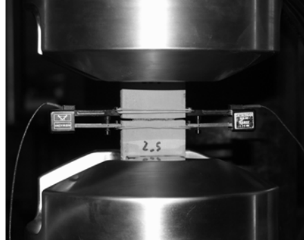
Fig. 2. Tensile test setup, including supports and clip gages.
