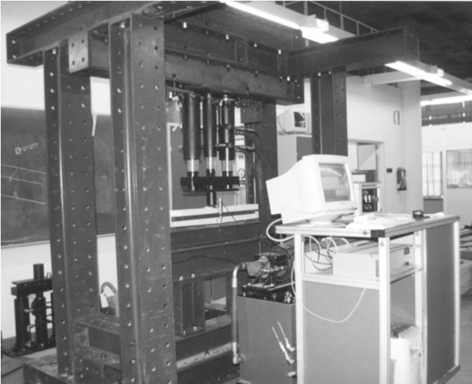
Figure 5 – Equipment and reaction frame.
