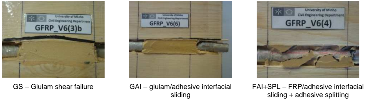
Figure 7 – Typical failure modes obtained
