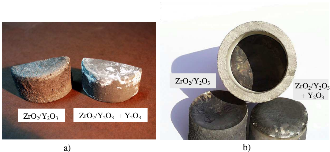
Figure 10 – Comparison between Ti-48Al samples obtained in single and multi-layer ZrO_2 based crucibles, revealing different metal-crucible material interaction
