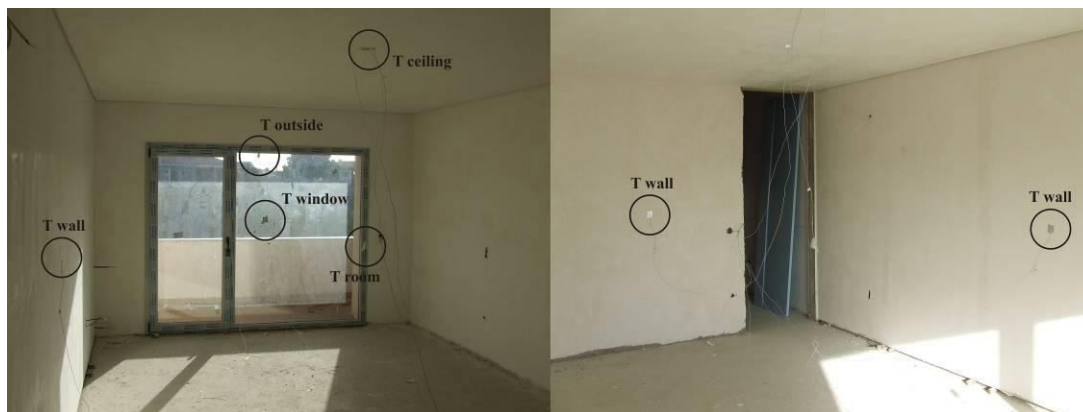
Figure 5.7.6. Schematic view of instrumentation placed (reference south room)
