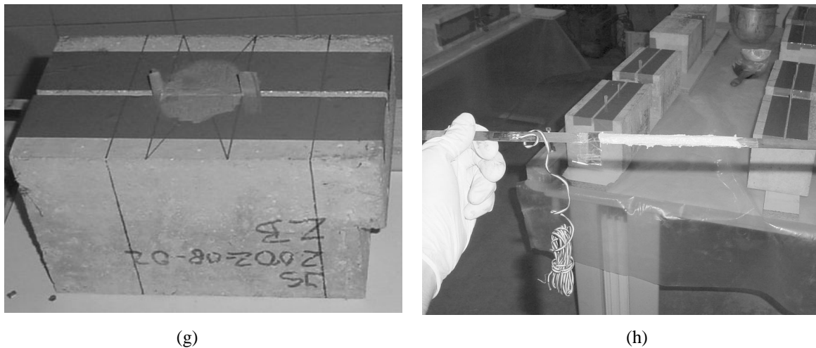
Figure 2.16 (cont.) – Specimen preparation: (g) slit filled with epoxy adhesive; (h) epoxy adhesive on the CFRP surface at the bond zone.
