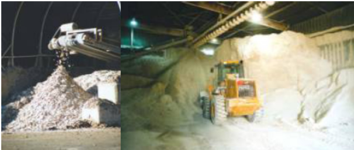
Figure 3.5. Plaster paper by-product, and final recycled gypsum product (WRAP, 2006).
