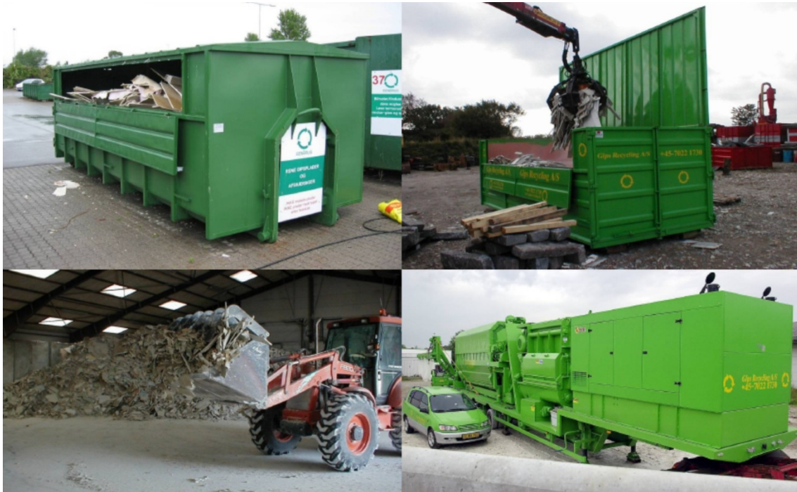
Figure 3.4. Recycling of plasterboard at Gypsum Recycling: collection, haulage, storage, and granulating (mobile unit) (WRAP, 2006a).
