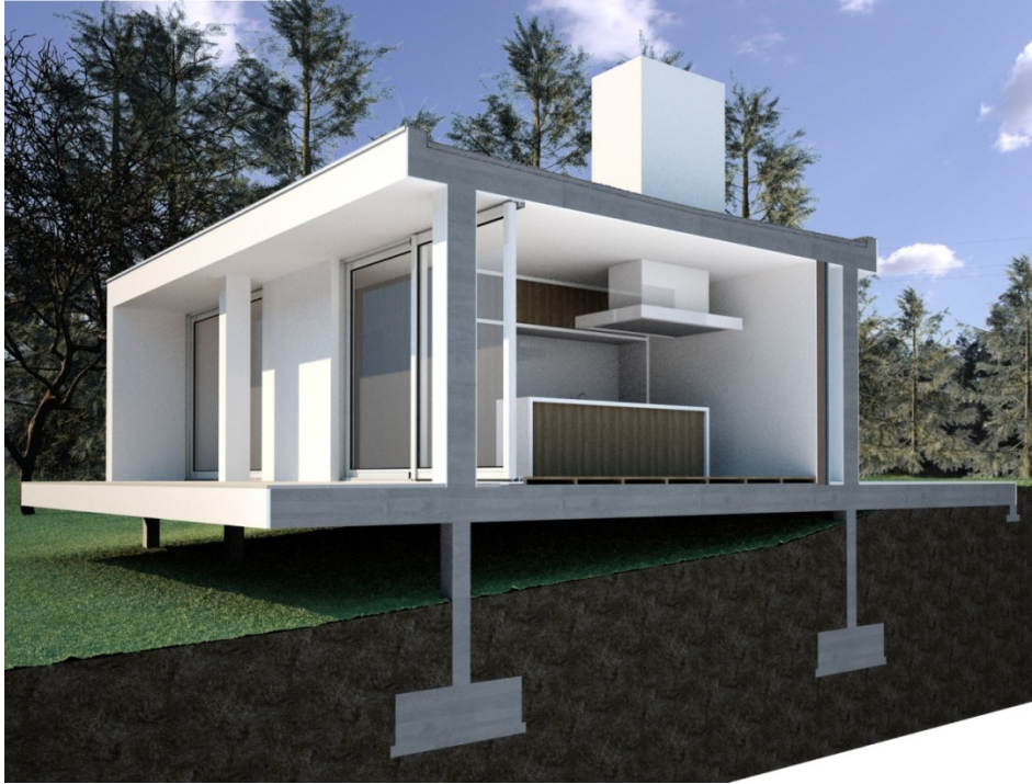
Figure 7.14. Building B1: 3D cross section.
