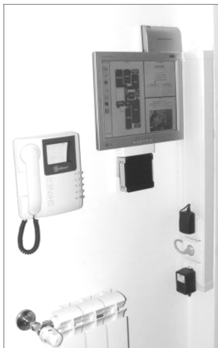
Figure 23 – User Interface console installation (control and feedback through a touch screen)
