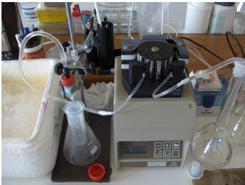
Figure 7. Nickel affinity chromatography was used for the purification of histidine-tagged recombinant human BMPs.
